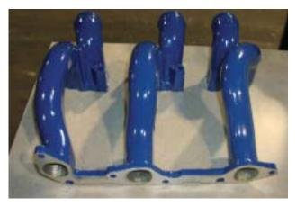
The intake manifold was Plaforized and then powder coated blue.
