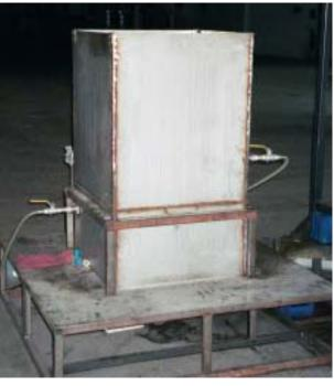
A small dip tank is used for Plaforization of parts at Smart Manufacturing, Schoolcraft, Mich.
