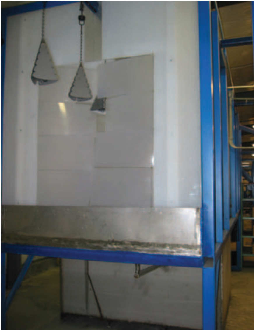
Parts enter the wash system by passing through polyethylene panels with slats cut into them.
