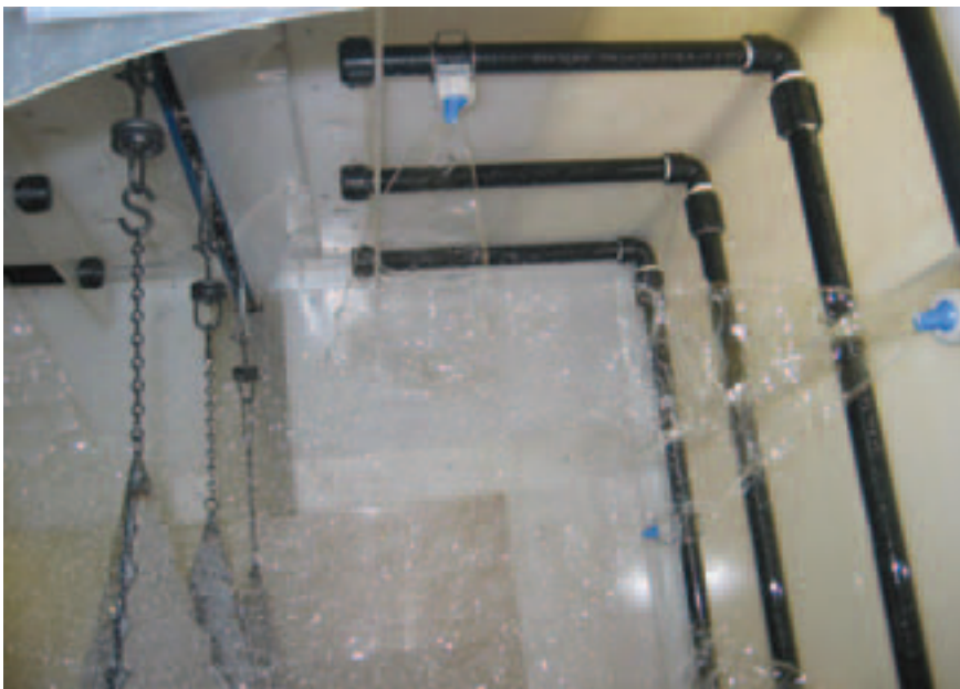
Spray nozzles apply the one-step nonaqueous cleaner to parts. A propylene glycol-based compound, the chemical cleans, phosphatizes, and seals metals without postrinses.
